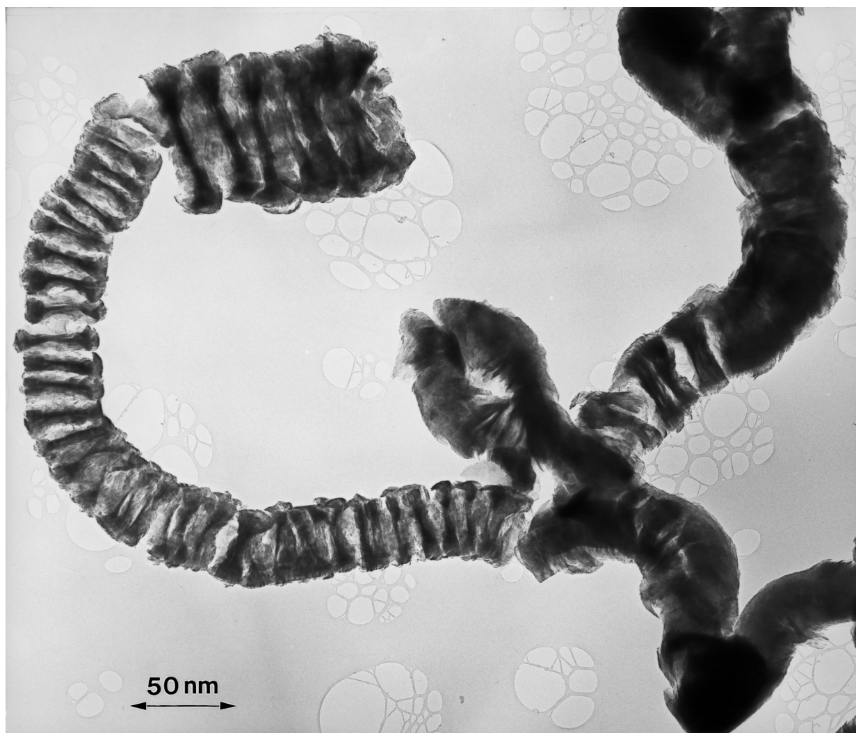
FIG. 6. Transmission electron micrograph showing the appearance of carbon filaments grown from the interaction of an Fe–Ni (7 : 3) powder with C_2H_4/H_2 (4 : 1) at 600°C.
